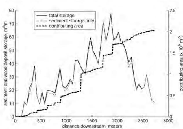
**Figure 10.** Cross-sectional areas of sediment and wood deposit storage averaged over 50-meter channel segments and samples every 20 years for the 3000 year simulation, and contributing area at 3000 years vs. distance downstream. Step-increases in contributing area occur at tributary junctions.
