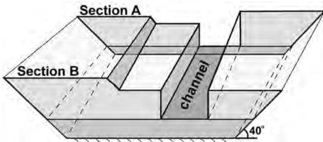
**Figure 6.** Schematic diagram of the sediment volume estimation method. Storage is calculated for sediment and wood both above the channel bed and including some sediment and wood below the channel bed in distinct wedges detectable from the longitudinal channel profile.
