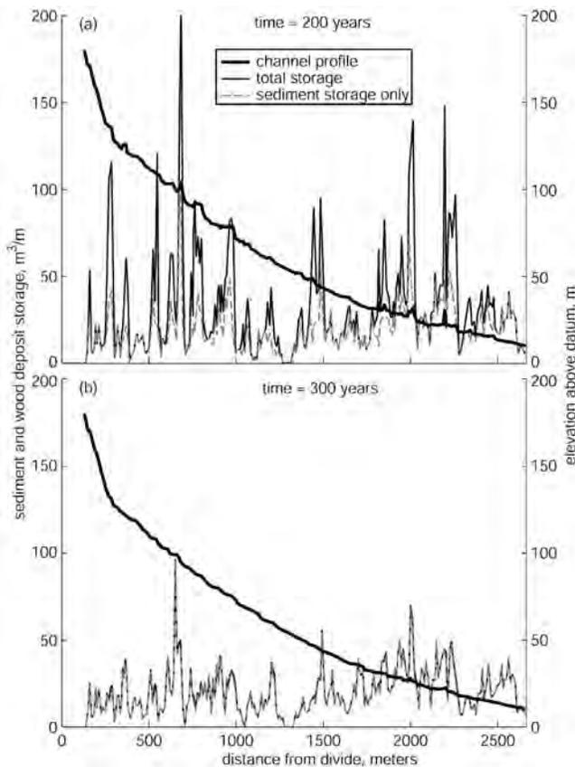
**Figure 8.** Simulated main channel profile and cross-sectional areas of sediment and wood deposit storage at every point along the main channel vs. distance downstream at two times, (a) 200 years (18 years after the first fire) and (b) 300 years (118 years after the first fire and before the second fire).
