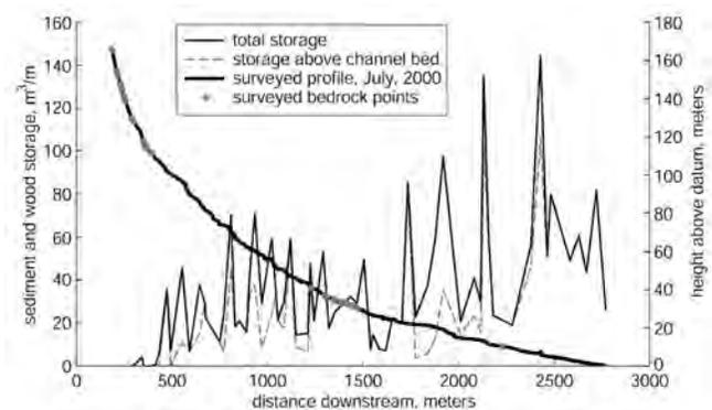
**Figure 7.** Surveyed Hoffman Creek channel profile with bedrock points highlighted and cross-sectional areas of sediment stored in surveyed valley transects vs. distance from divide. Two storage estimates are shown: sediment stored above the channel bed, representing a minimum estimate; and a more realistic estimate including sediment “wedges”.
