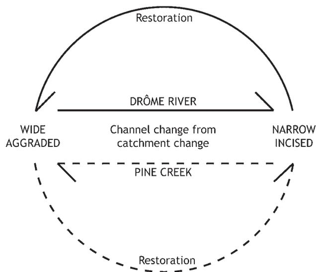
**Fig. 1** Contrasting directions of channel planform evolution due to changes in catchment sediment yield, and consequent directions of intended restoration in Pine Creek, Wyoming, USA and the Drôme River, southern France (From Kondolf *et al.*, 2002; with permission from Elsevier).
