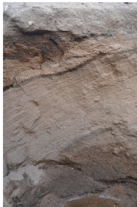
FIGURE 3 | Alternating layers of fine and coarse sediments within a sand dam deposit (Viducich 2015).
