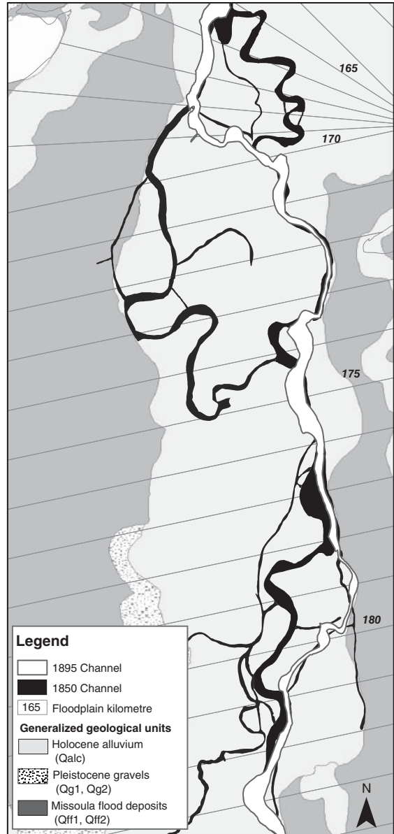
Figure 25.9 Example of avulsions 1850–1895 along upper Willamette River. Similar large-scale avulsions occurred along the entire Willamette River during this time period. In many cases, the 1895 channel avulsed into former side channels (e.g. FPKM 165–170) or carved cut-off channels (e.g. FPKM 169). Geological map from O'Connor et al. 2001. Historical Willamette River channel maps and floodplain transect maps from Hulse, Gregory, and Baker 2002.
