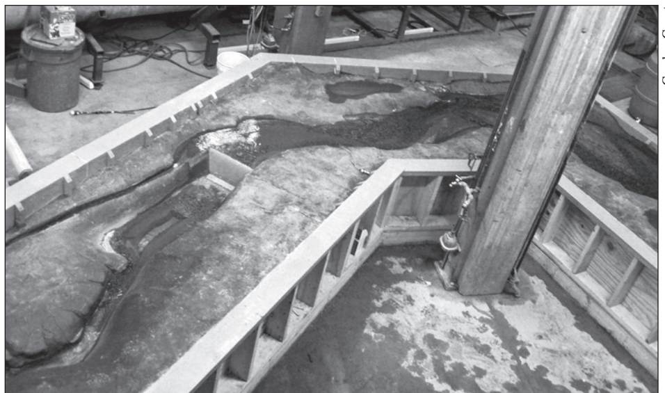
A scale model allowed the researchers to test if notching the cofferdam would affect the pattern of reservoir sediment erosion.
