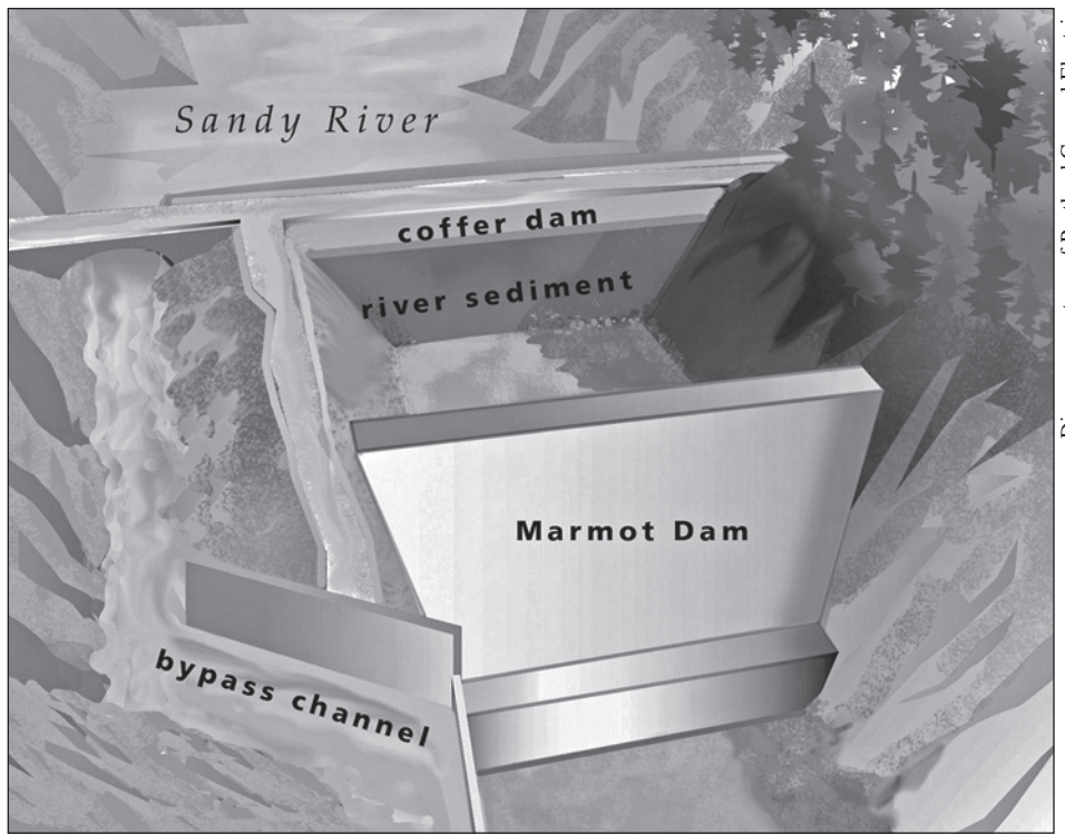
A temporary cofferdam upstream of the dam diverted the river to a bypass channel while work crews removed the concrete structure.
