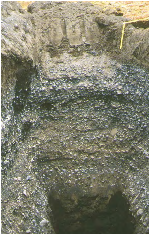
Fig. 14. Detail of fluvial sediments which occur immediately below the ‘main’ surface at all locations. Section is into a test pit; uppermost layer is soil. The thickness of the fluvial unit is 4 m at this location. The laminated fine sand which underlies the fluvial sediments is separated by an extensive erosion surface.
