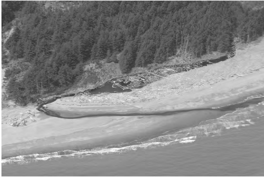
Fig. 3. Sand-filled LWD deposit diverting stream discharge to form a backshore lake to the north of study site three. Outflow channel on beach is \sim 3 m wide for scale. Photo credit: K.I. Pearce.
