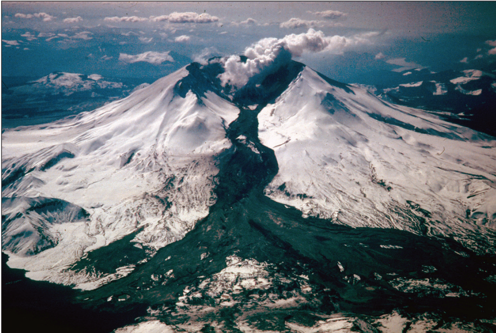
Figure 2-13—Oblique aerial photograph of March 1982 snowmelt-triggered lahar. View to south. The flow originated after a water flood from the crater entrained sediment along the steep north flank and increased its ratio of solids to fluid. Most of the flow traveled west (right) down the North Fork Toutle valley, but a substantial fraction flowed into Spirit Lake (on left). U.S. Geological Survey, March 21, 1982.
