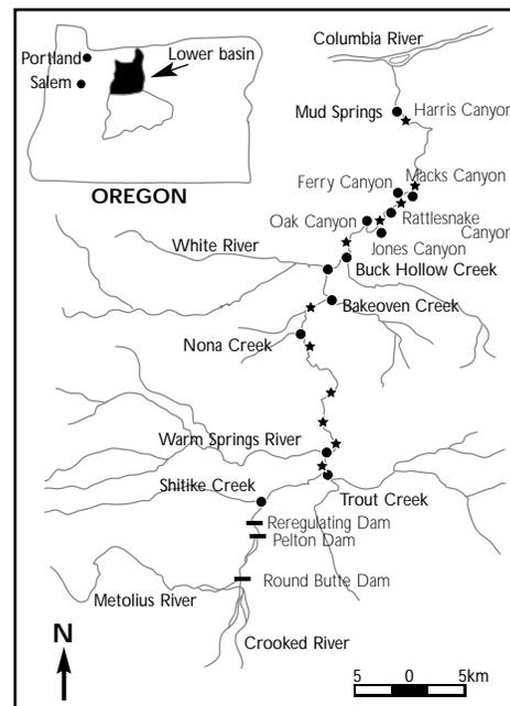
**A** Map of three dams in the lower Deschutes River basin: Round Butte Dam impounds Lake Billy Chinook, which holds over 40 percent of the water stored in the Deschutes basin. Just downstream is Pelton Dam, responsible for daily peaking power production, then the Reregulating Dam, which provides constant discharge to the lower Deschutes River, evening flow on a daily basis.
