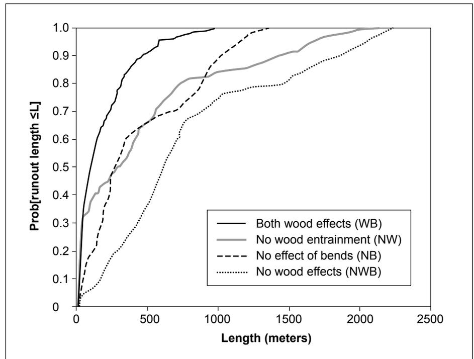
Runout length distributions simulated by the physics-based debris flow model, with and without wood.
