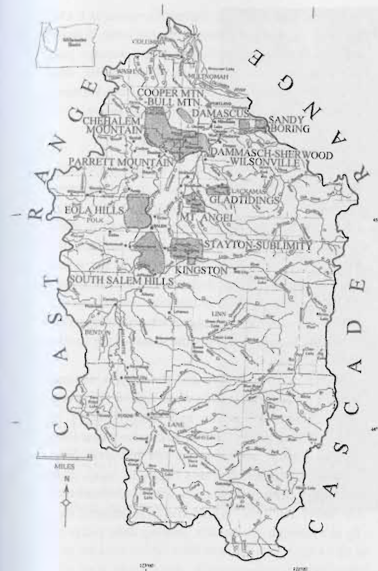
The state Water Resources Department has designated 22 regions throughout Oregon as areas where the amount of groundwater is depleted. Of these, 17 draw from the interbeds of the Columbia River Basalt Group in the northern Willamette basin (shown in pattern), and the remainder are located in eastern Oregon. The department can impose restrictions on future use where drawdown from the aquifer exceeds the estimated natural long-term recharge rate. (After Bastasch, 1997; Burt, et al., 2009; Oregon Water Resources Department, 1984, 1992; Orr and Orr, 2005).
